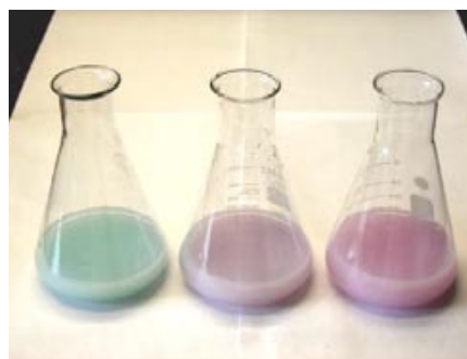
Figure 2 Same colour changes for magnesium chloride back-titration as in Figure 1, but for cloudy (opaque) sample solution, eg milk. Left flask: blue colour well before endpoint. Centre flask: last trace of blue/purple. Right flask: pink/red colour at endpoint
