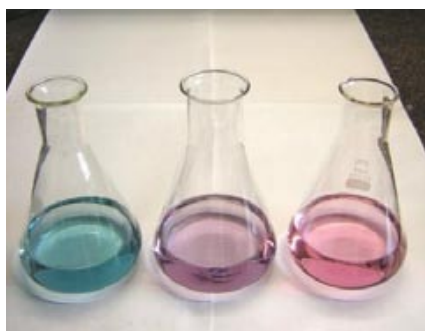
Figure 1 Colour changes for magnesium chloride back-titration in clear solution using Eriochrome Black T indicator. Left flask: blue colour well before endpoint (all Ca^{2+}/Mg^{2+} ions complexed by excess EDTA, all indicator molecules uncomplexed). Centre flask: last trace of blue/purple colour just before endpoint (excess EDTA almost totally complexed by added Mg^{2+} ). Right flask: pink/red colour at endpoint (all EDTA complexed by added Mg^{2+} , indicator also complexed).
