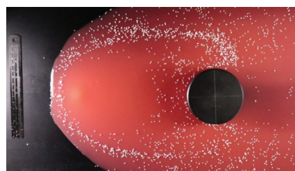
View from above of the flow of PEG600 down an inclined plane and around an obstruction. Buoyant makers are visible and enable the reconstruction of the free surface velocity field.
