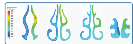
Total pressure contours at nasal cavity cross-sections 15, 30, 45, and 60 mm (left to right) from cannula with NHF at 30 L/min.
