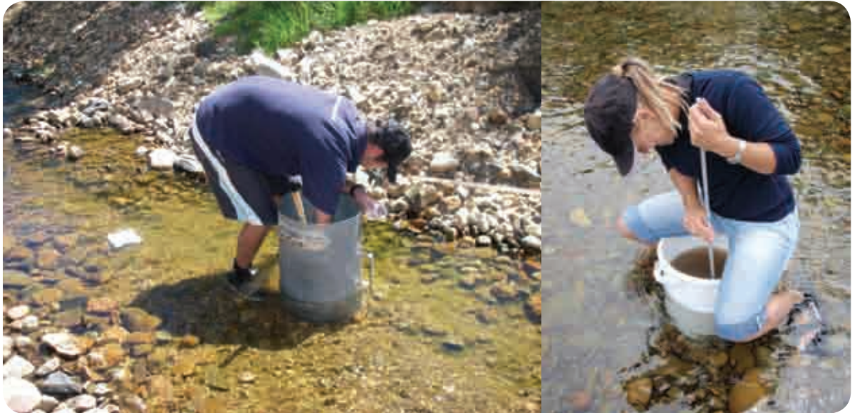
Figure 4-4. Photos of sample collection using the Quorer method.
