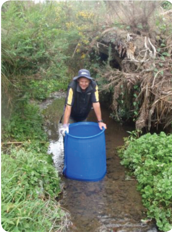
Figure 4-18. Large corers successfully applied to extend the physical limitations of the Quorer method.
