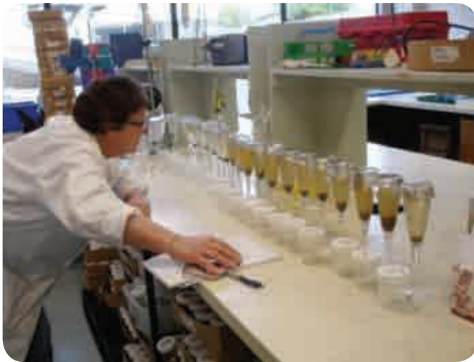
Figure 2. Reading settled volumes on multiple samples from contrasting sites from Whatawhata Research Centre streams.
