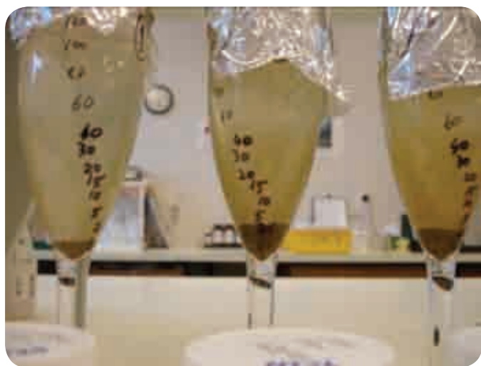
Figure 1. Graduated acrylic champagne flutes used to measure settled volume of Quorer method samples.
