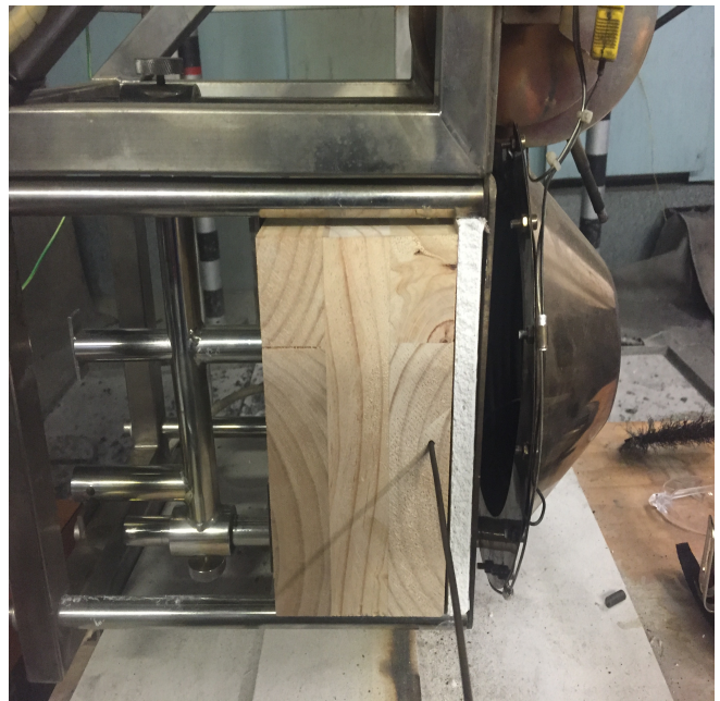
Figure 1. CLT sample with a Magnesium Oxide lining pictured before commencement of testing
