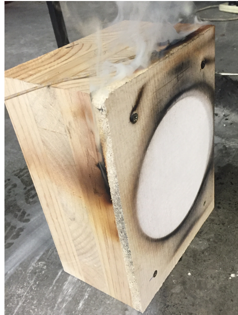
Figure 1 sample of CLT with 12 mm Magnesium Board lining pictured at completion of 65 \text{ kW/m}^2 test
