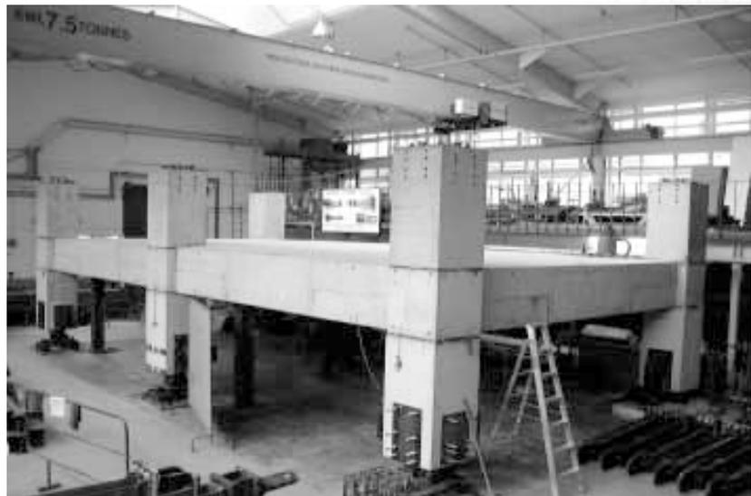
*Test specimen ready for load frames to be attached*
