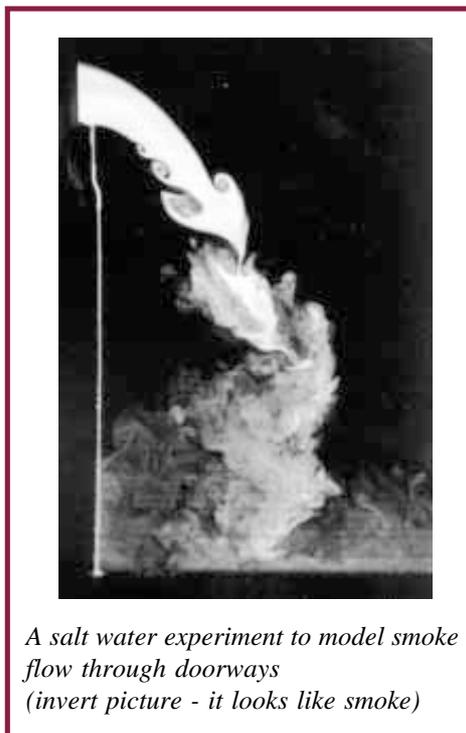
*A salt water experiment to model smoke flow through doorways
