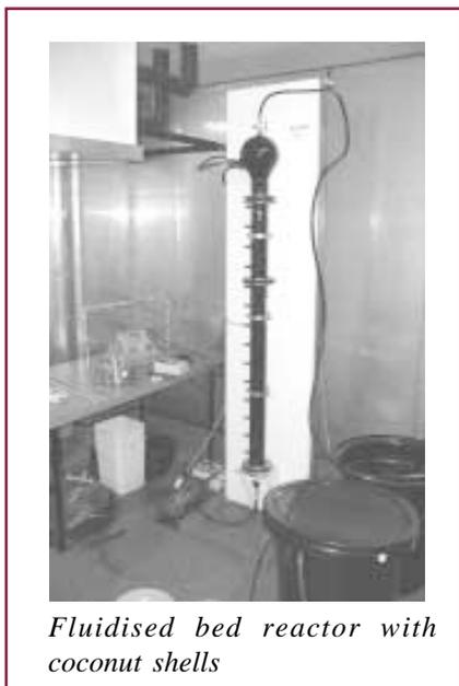
*Fluidised bed reactor with coconut shells*
