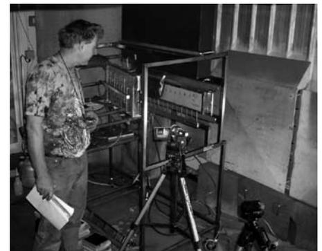
Geoff Merryweather observes flame spread tests over timber samples in the LIFT apparatus
