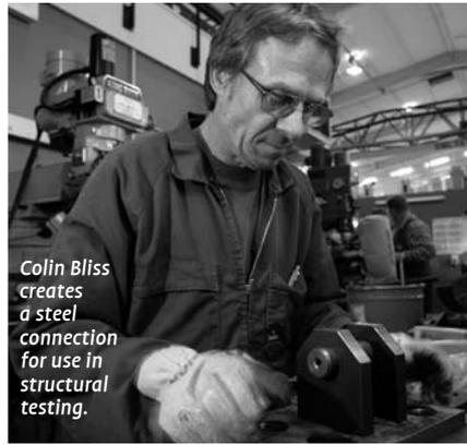
Colin Bliss creates a steel connection for use in structural testing.
