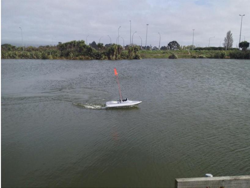
**Appendix 1.** The remote controlled jet boat used to gather bathymetry data
