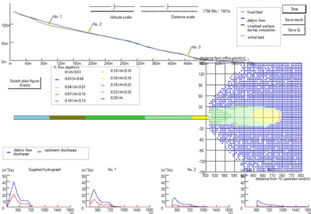
Figure 10 - 2d model showing area of debris deposition from main channel.
