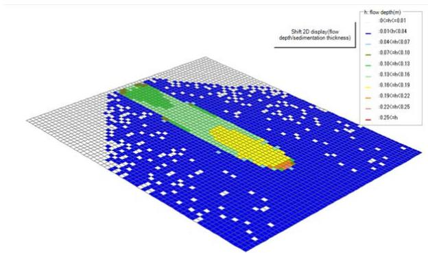
Figure 8 - Extent of a debris flow from the secondary channel
