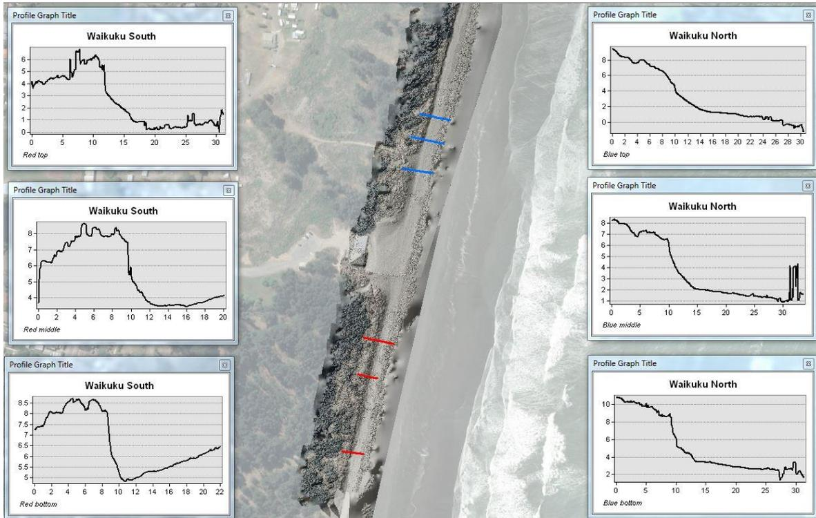
**Figure 7:** Digital Surface Model of both **Waikuku North** in blue, includes Beach-profiles. Includes the warped data of **Waikuku South**.
