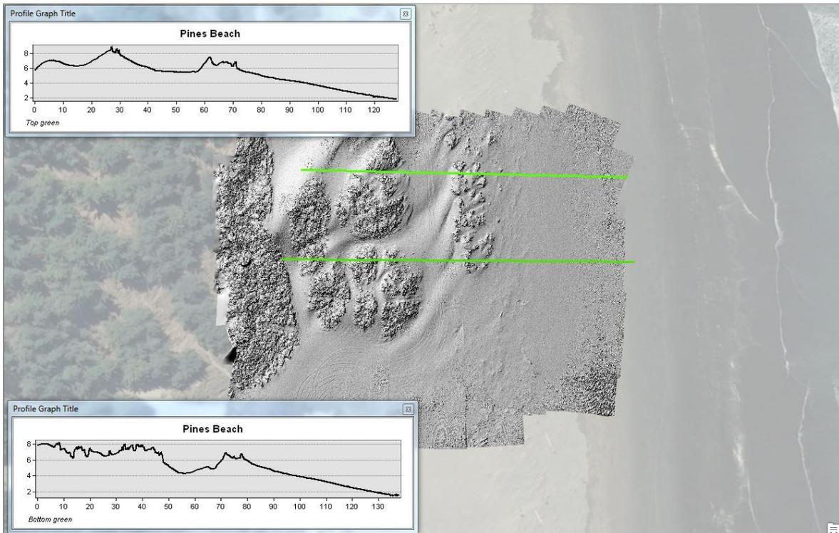
**Figure 6:** Digital Surface Model of **Pines Beach** with upper and lower transects and Beach-profiles.
