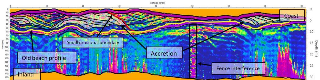
**Figure 11:** Processed and interpreted GPR data acquired at Pines beach, (100MHz antenna). Red represents erosional surfaces while the white shading represents areas of accretion.
