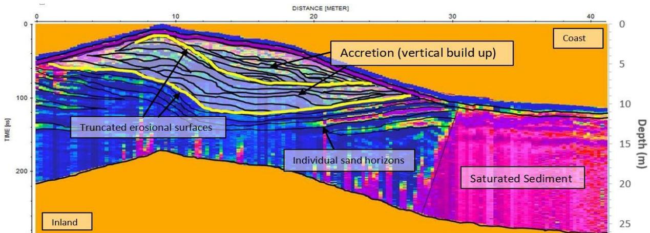
**Figure 12:** Processed and Interpreted GPR data acquired at Waikuku beach, (100MHz antenna). The yellow lines indicate erosional surfaces while the white shading represents accretion.
