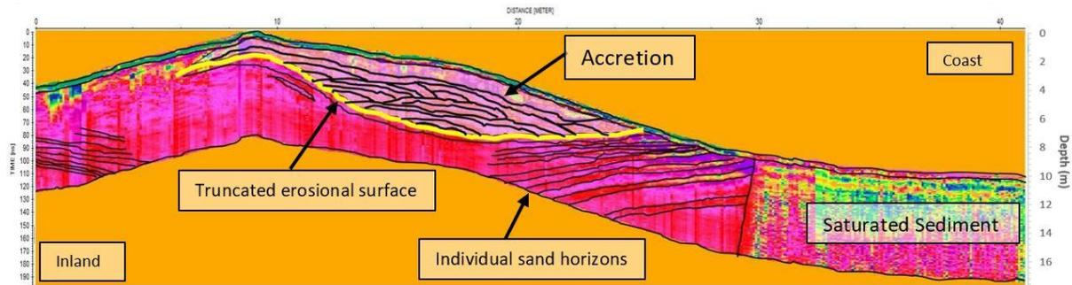
**Figure 13:** Processed and Interpreted GPR data acquired at Waikuku beach, (200MHz antenna). The yellow line represents an erosional surface, while the white shading shows areas of accretion.
