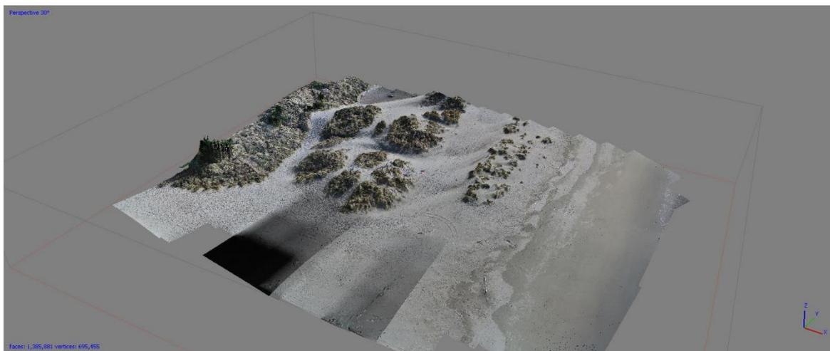
**Figure 4:** Dense Point Cloud model with mesh of **Pines Beach** in Agisoft.
