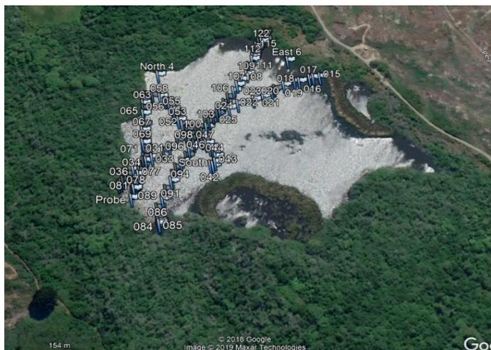
Figure 3: Tūtaepatu Lagoon waypoints showing transects conducted using a kayak and depth probe
