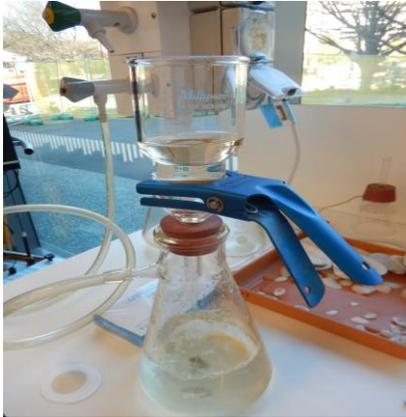
Figure 4: Removing sediment from water sample in Geography laboratory using vacuum pump
