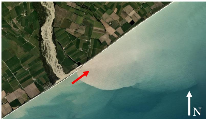
**Figure 23.** Aerial image showing long-shore transport of sediment in a south to north direction, indicated by red arrow. This is moving sediment away from the southern end of the RRME and towards the northern end, which could be contributing to erosion in the south and accretion in the north. Image sourced from *Planet Labs*.
