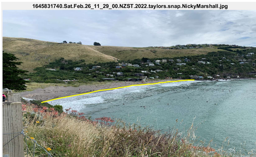
Figure 8: Shoreline Plot at Taylors Mistake, Christchurch, New Zealand on Sunday 26 th of February at 11:29am. Shorelines were created on MATLAB using the CoastSnap code produced by Mitchel Harley.
