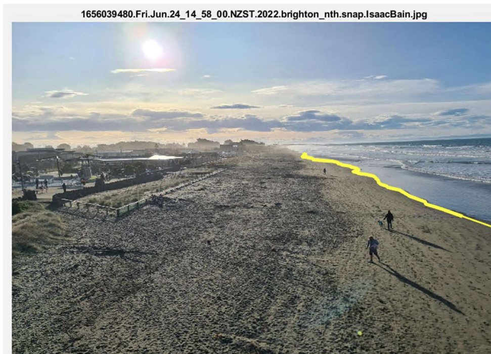
Figure 9: Shoreline Plot at New Brighton, Christchurch, New Zealand (North) on Friday 24 th of June at 14:58. Shorelines were created on MATLAB using the CoastSnap code produced by Mitchell Harley.
