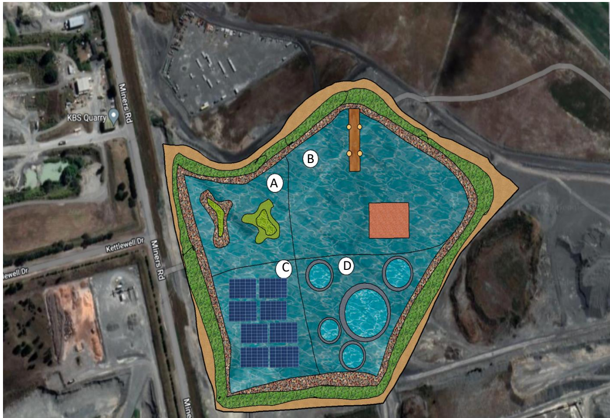
Figure 9. Schematic drawing showing potential uses for a quarry waterbody. (A) Ecological waterbody, (B) Recreational waterbody, (C) Floating Solar Arrays, (D) Aquaculture.
