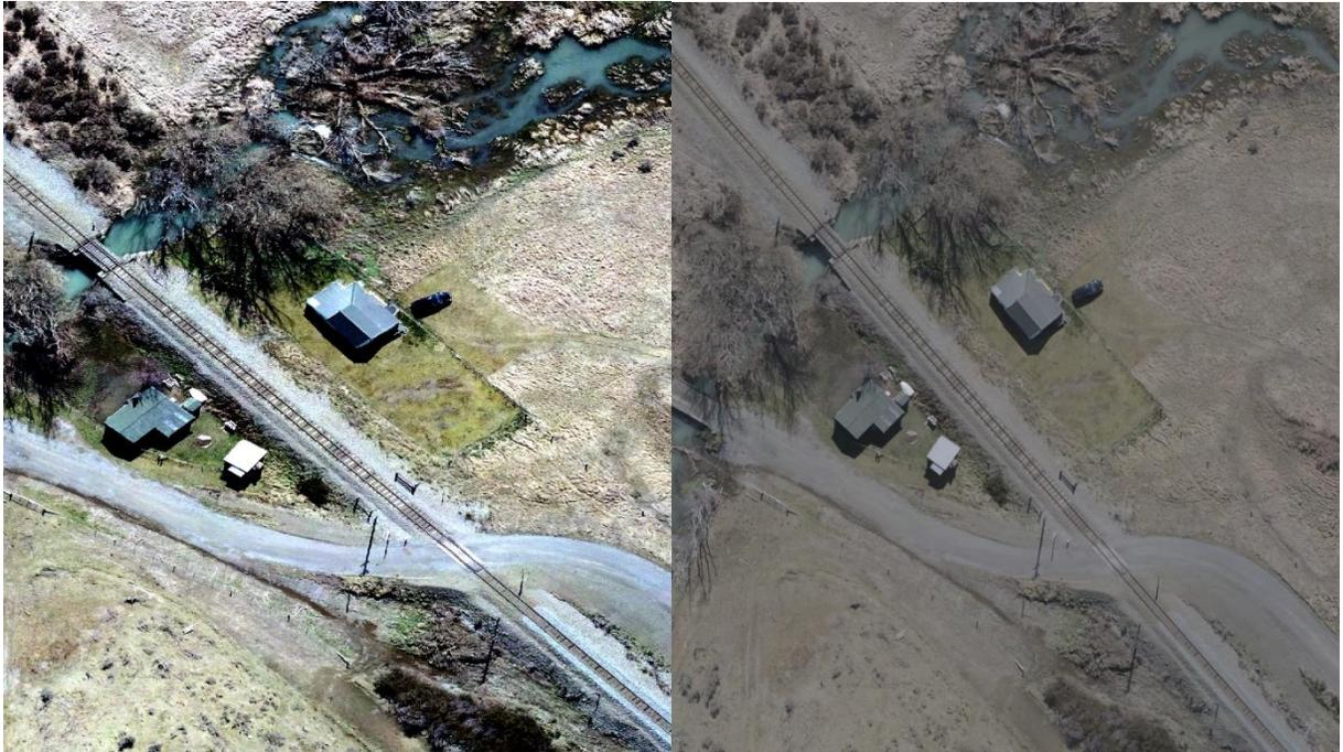
Figure 11. Distortion caused by different projection systems. Note the roof of the buildings, the buildings in the left image (WGS 1984) are not at right angles (distorted) while the building in the right image (NZGD2000 / UTM zone 59S) are (normal).
