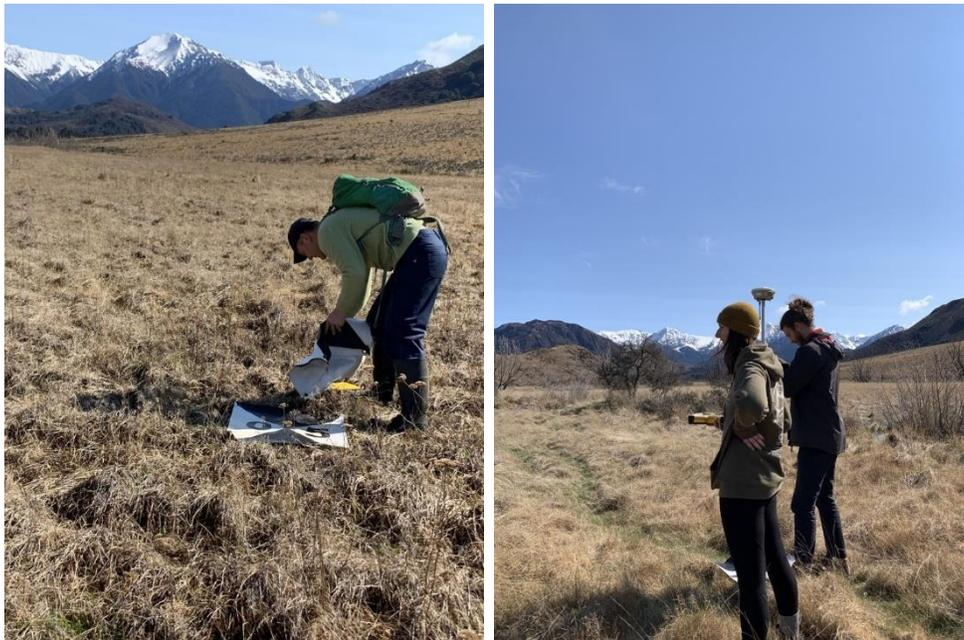
Figure 3 & 4. Images of data collection at the site. Figure 3 shows the placement of a GCP and Figure 4 shows the GCPs' GPS coordinates being logged.
