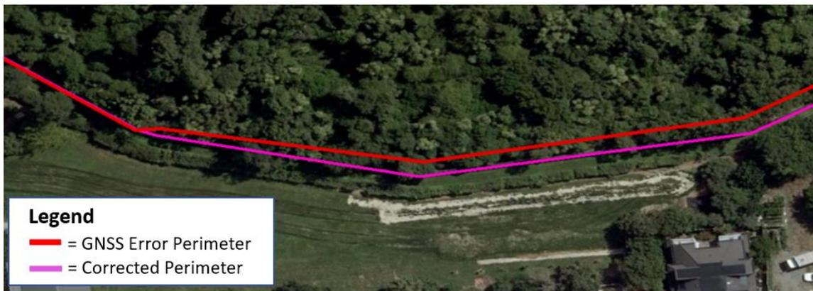
Figure 4: Showing GNSS error data of the perimeter fence compared against the satellite corrected perimeter fence
