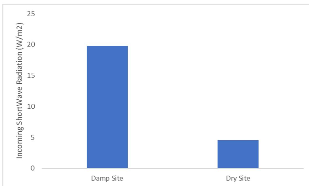
Figure 5. Mean incoming shortwave radiation from the weather stations in the damp site versus dry site at Riccarton Bush.
