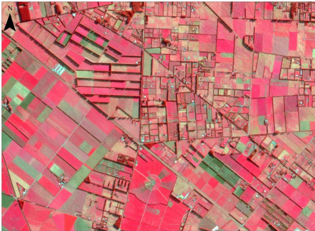
Figure 3) A segment of the wider Canterbury infrared image. This image was obtained from Planet Labs which contains the 2, 3 and 4 wavelength bands. Bright red areas show healthy vegetation, and bright green areas show unhealthy vegetation. Grey or white area represent non-vegetated surfaces including roads, or buildings. This near-infrared image is highly useful for detecting vegetation health and land use patterns when completing classification.
