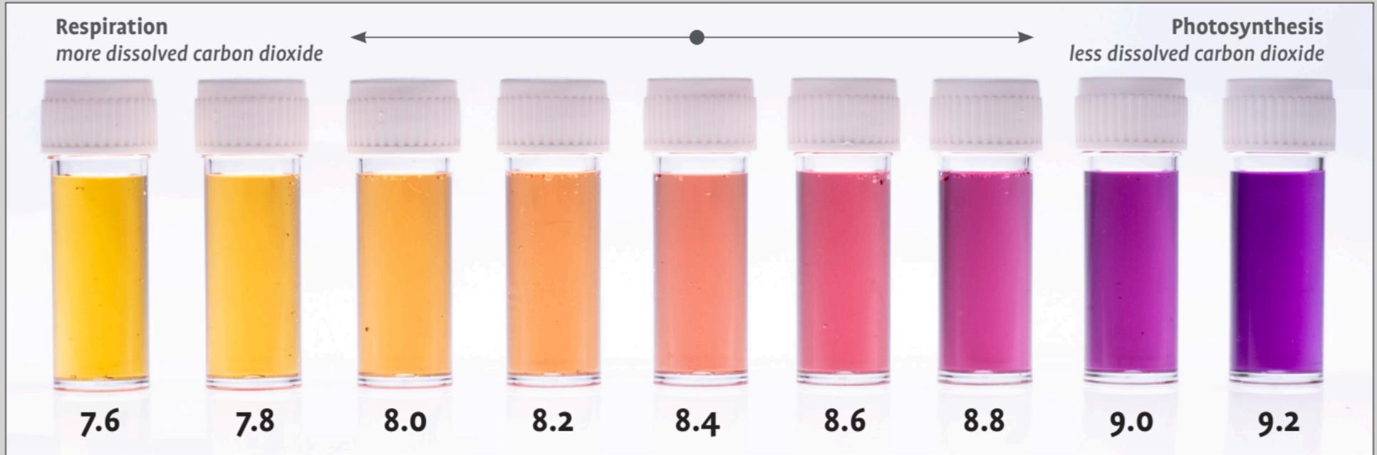
Note: Hold samples in front of a bright white light source to obtain accurate measurements.
