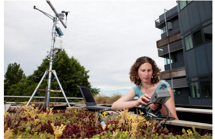
Frances Charters, a PhD student, viewing the Living Roof trial at Civil and Natural Resources Engineering: one method to improve storm water quality
