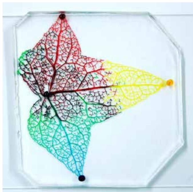
The resulting ivy leaf photomask (left), produced by depositing a thin film of chrome onto the leaf nervature coated with photoresist, and (right) the microfluidic platform, filled with four different dyes.
