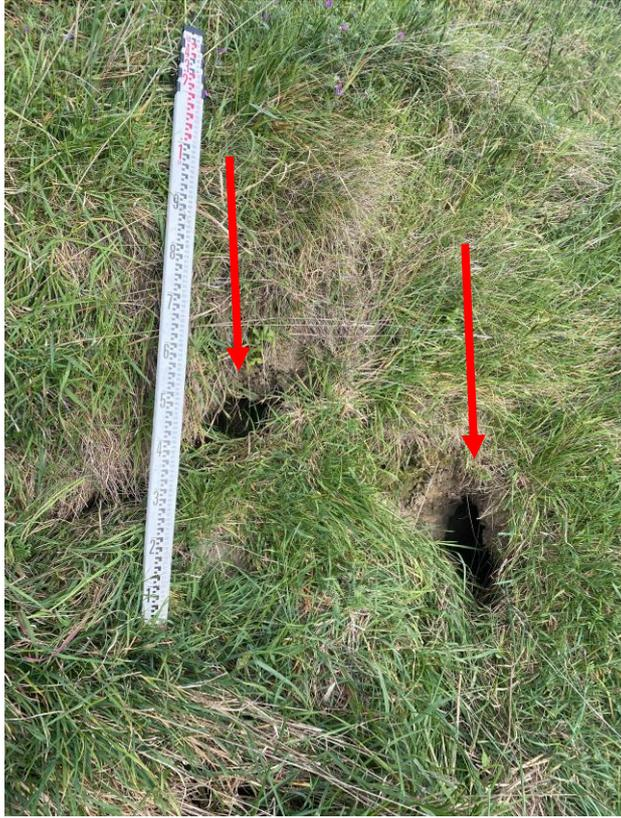
Figure 11: Tunnel Gully Holes at Mt. Vernon, Indicated by the Red Arrows. The Measuring Staff is 1 m for Reference.
