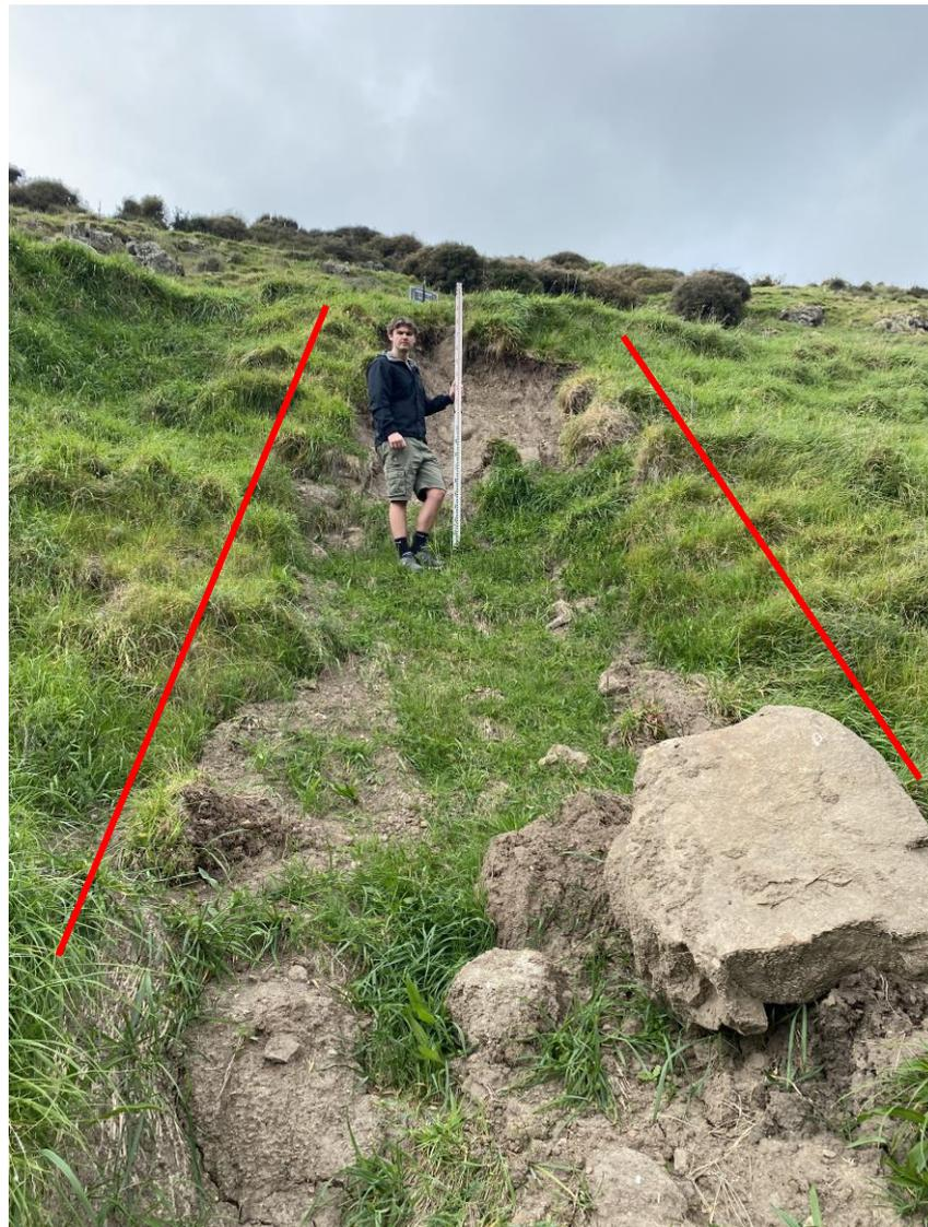
Figure 14: Mass Movement at Mt. Vernon, Indicated by the Red Lines. The Measuring Staff is 2 m for Reference.
