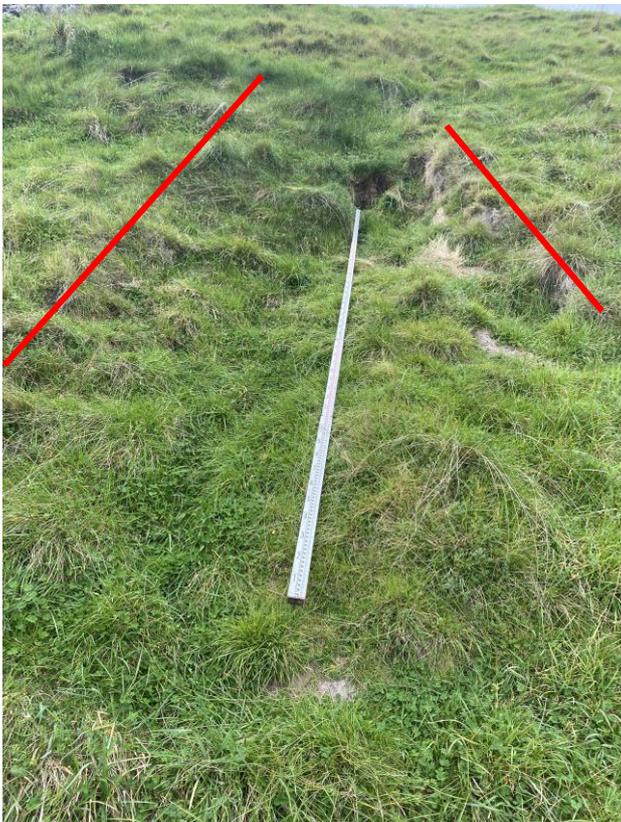
Figure 12: Collapsed Tunnel Gully Erosion at Mt. Vernon Park, Indicated by the Red Lines. The Measuring Staff is 5 m for Reference.
