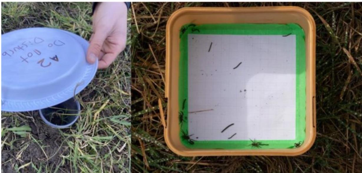
*Note.* Left: Trap A2 at Site A showing the trap roof (plastic plate) and trap cup used to capture GDI. Right: An ice cream container lined with graph paper was used to count and identify specimens in the traps.
