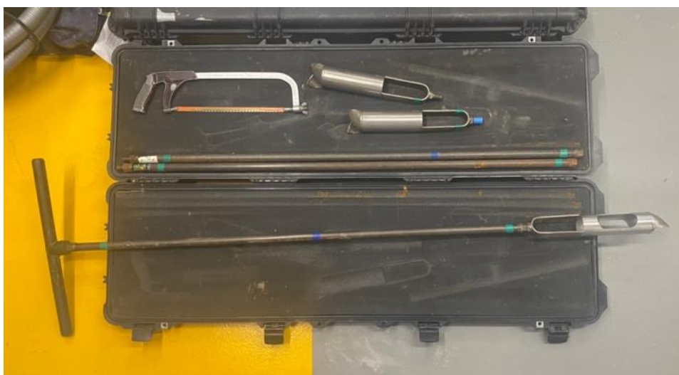
Figure 4. Hand Auger used in second phase of sampling.
