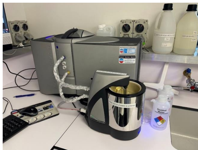
Figure 7. Mastersizer Hydro LV 3000 that was used.
